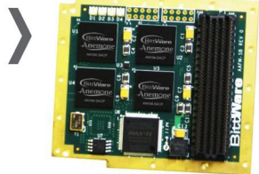
Figure 3 | FMC board with four floating-point coprocessors for FPGAs
