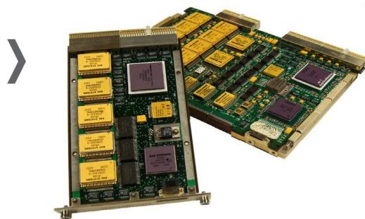
Figure 1 | RAD750 single board computers from BAE Systems come in 3U and 6U form factors.
