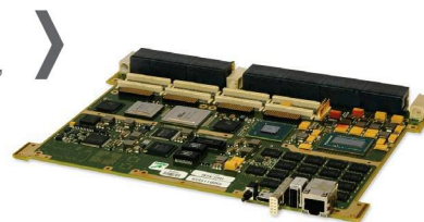
Figure 1 | The SBC625 from GE Intelligent Platforms, a 6U VPX board using Intel's 2.3 GHz Core i7-3615QE processor
